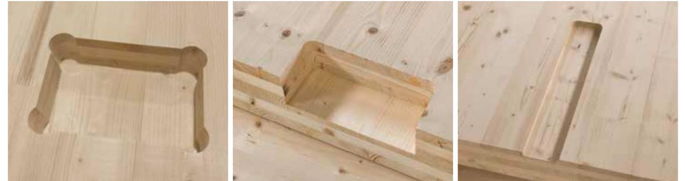
We use an end mill or cylindrical mill cutter to create slots – recesses with a limited depth – for example to inlay steps in a staircase or to mount steel brackets and connectors. These elements can also be rounded depending on the tool used.
