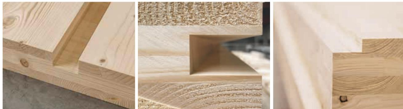
Full-length milling on the surface and front side as a rebate can be done with different thicknesses and depths, for example as a groove on the front side for a tongue on a separate piece.
