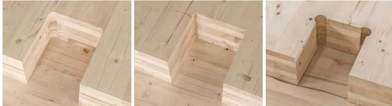
Whether you need recesses for purlins or rafters, outlets for heating / ventilation / sanitation facilities or window or door openings, an end mill can be used to design all kinds of outlets and openings. Corner cut-outs made with an end mill are usually round to begin with, but they can also be given sharp edges or milled diagonally.
