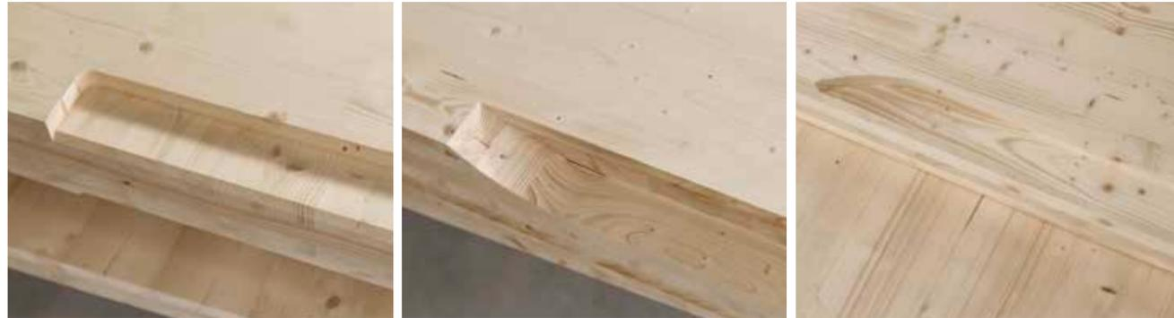
We create a limited rebate using the cylindrical mill cutter or end mill. Round shapes can also be created here depending on the tool used.
