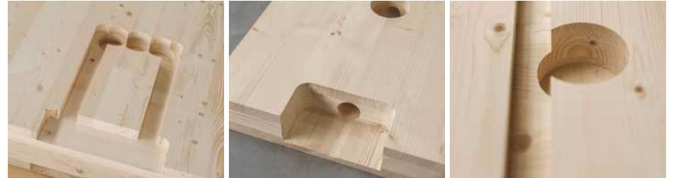
Holes can be drilled for cable ducting, sockets, as a pilot hole for subsequent screw connections, and other uses. We can use a 32 mm deep-hole drill to create electrical ducts inside visual-quality wood products.
